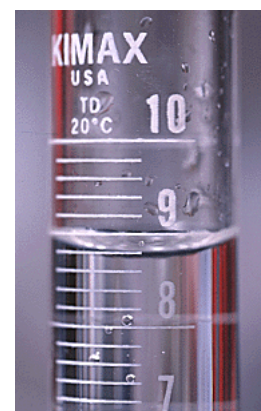
The volume of water in this cylinder would be read as 8.8mL, not 9.0mL.
